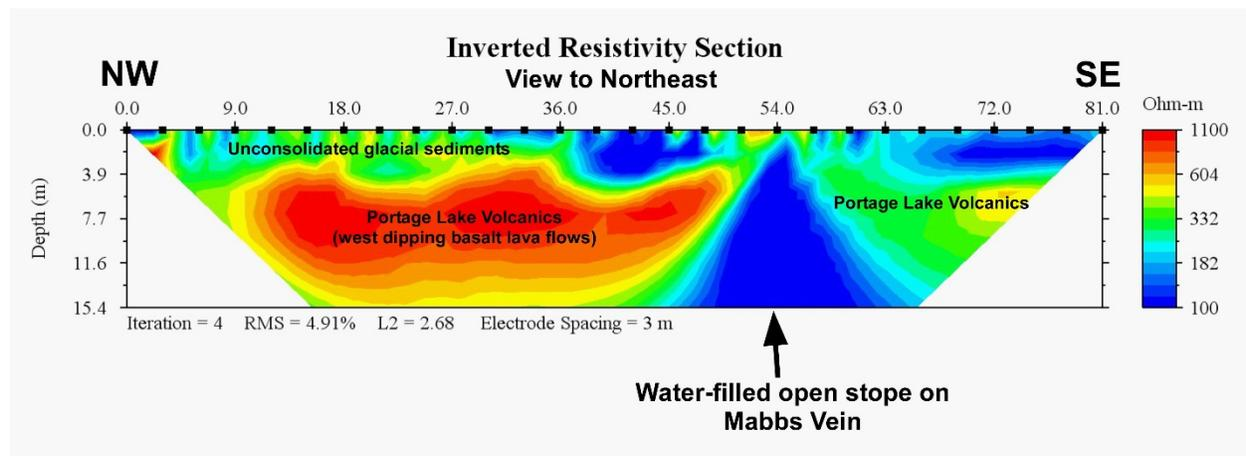
Figure 8: Resistivity section across the Mabbs Vein approximately perpendicular to the strike of the vein and host basalt lava flows about 20 ft from the southwest corner of the main museum building (see Figure 1). The geophysical measurements and contouring were completed by Michigan Tech students as part of an intensive summer course in field geophysics taught by Dr. Jeremy Shannon.
