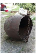
Kibble, barrel-shaped,  $\sim 3\,$  ft. high and 2.5 ft. across top opening, an estimated weight of 250 lbs.
