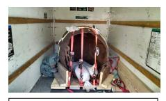
Kibble strapped to a wood base with sides wedged. Base strapped to corners and wedged against side of the trailer to avoid sliding. Weigh added to avoid tipping
